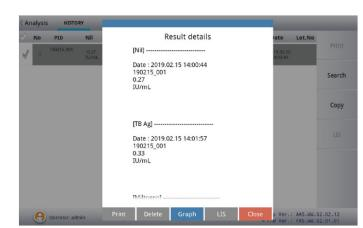
9. Press the "History" to make sure the test results. Each result can be popped up when press the result for 3 to 5 seconds.
