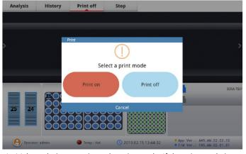
4. Make a choice to activate the print mode. If the print mode is on, the results of 3 tubes per a specimen are printed out when 3rd (Mitogen tube) test is finished.
