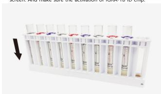
3. Load the processed tubes into the tube rack sequentially.
