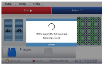
6. Clean out the remaining tips and cartridges used in the trash bin. \* Make sure the tip ejecting area is empty.
