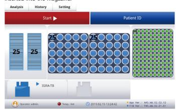
2. Adjust the number of test cartridges, tubes and tips on the touch screen. And make sure the activation of IGRA-TB ID chip.
